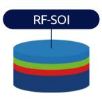
Reference substrate for smartphone RF FEM (LNAs, Tuners, Switches)
